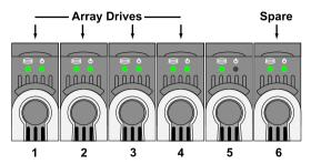
In the example above, there is a four-drive RAID 5 disk array and a global spare drive. Physical drives 1, 2, 3, and 4 belong to the disk array. Physical drive 5 remains unconfigured. Physical drive 6 is a revertible spare drive.
